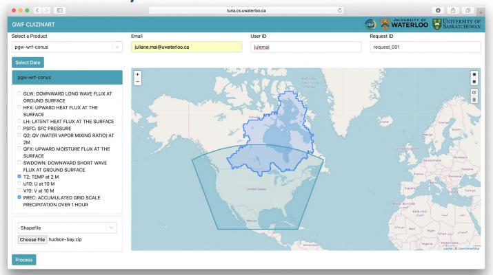
Frontend of GWF Cuizinart with domain selected by shapefile upload (or GeoJSON or drawing)
