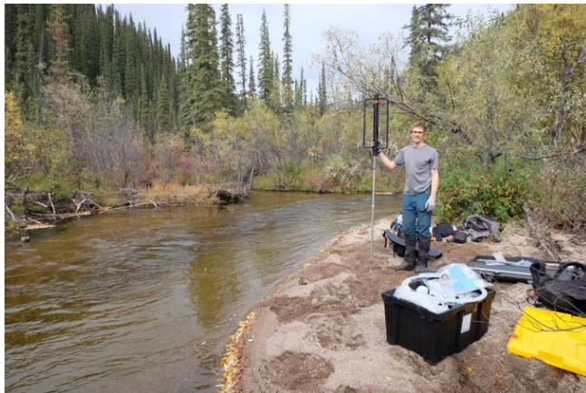
FDr Skierszkan installing drive-point piezometers for groundwater sampling on traditional territory of the Tr'ondëk Hwëch'in First Nation (Dawson Range, Yukon, Canada)
