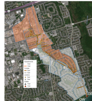
Figure 2. Layout of two modeled Ajax sewersheds where the blue lines identify the sub-basin boundaries, orange and gray circles are stormwater collection nodes, orange and white lines are the main sewers, red and gray triangles (OW and OE) are the stormwater outfalls of the two sewersheds.
