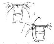
5. Pull the ends of the wire to close the bag. Holding the bag by the wire ends, whirl the bag three complete revolutions to form a leakproof seal. Whirling the bag Will form the tightest seal. Larger bags can be closed by "folding" the tab over as tightly as possible.
