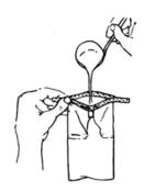
4. Put sample, liquid or solid, into bag. Leave enough space at the top for closing and mixing if needed.
