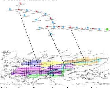
Schematic of coupling location between WATFLOOD and MODSIM models of Lower Nelson River Basin
