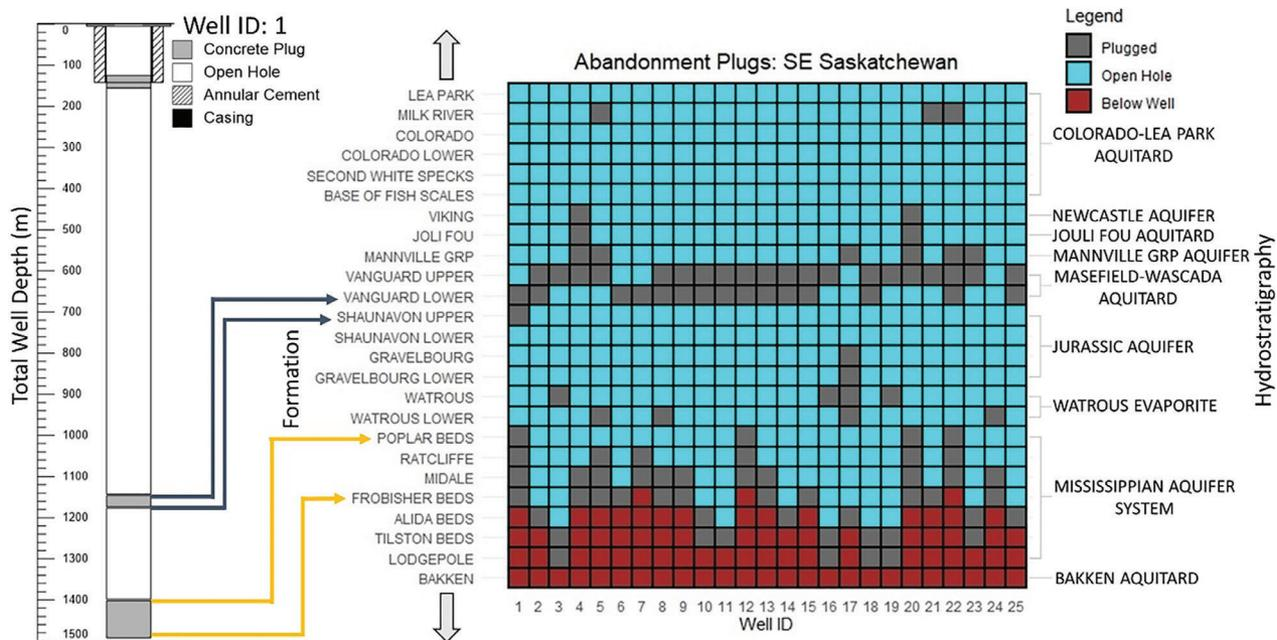
Figure 5. An example of a typical well abandonment schematic for a drilled and abandoned well on the left with plug placements in old abandoned wells on the right for the Southeast Saskatchewan study area.
