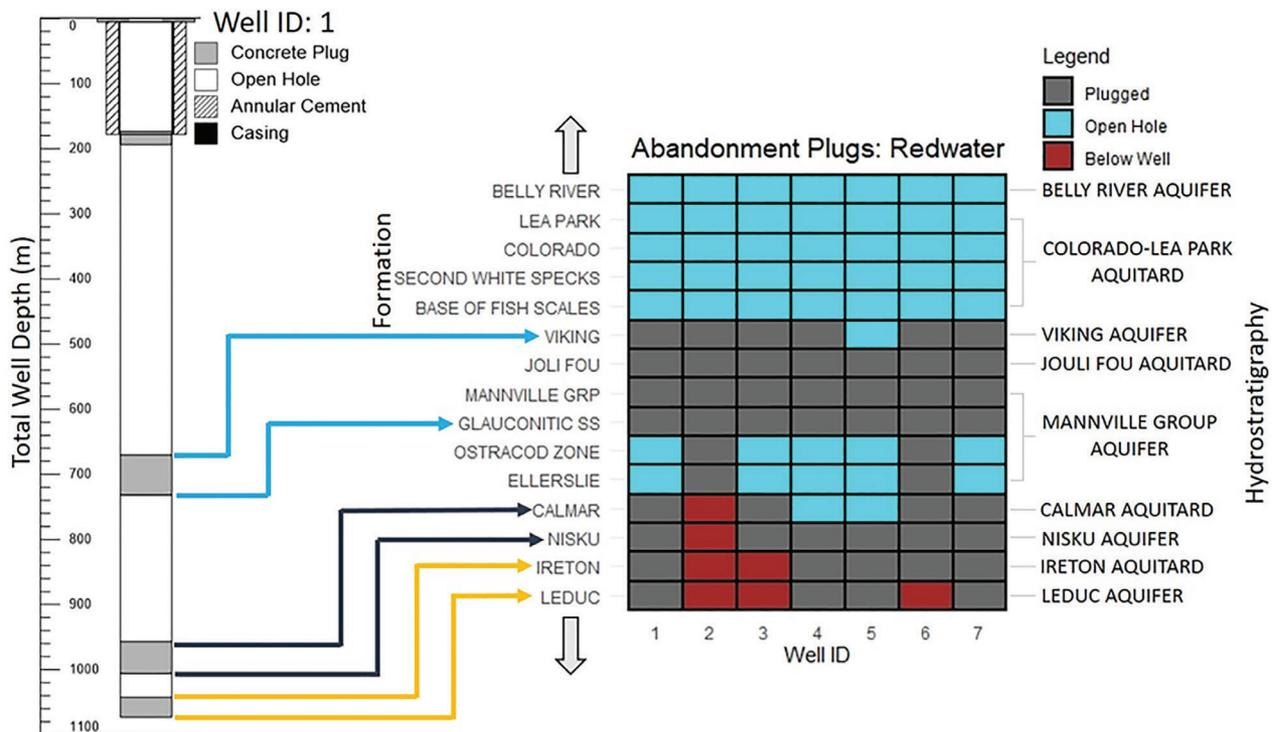
Figure 6. An example of a typical well abandonment schematic for a drilled and abandoned well on the left with plug placements in old abandoned wells on the right for the Redwater study area.
