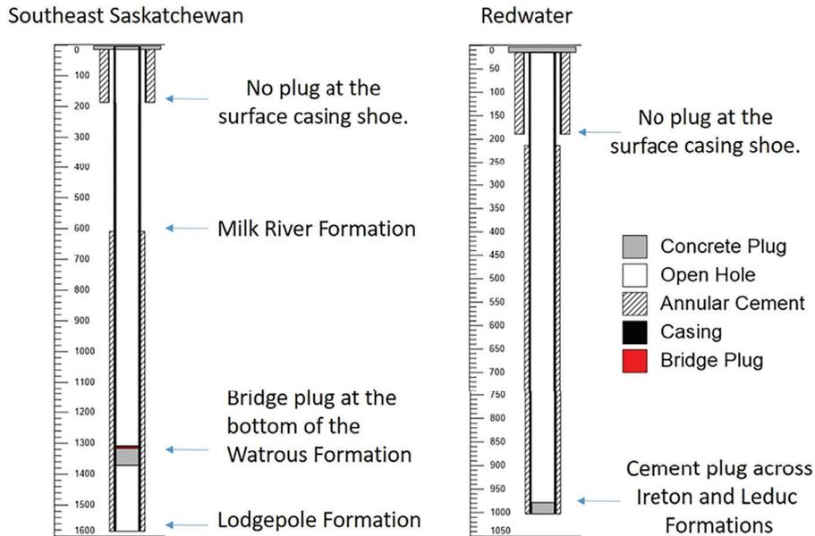
**Figure 8.** Cased well abandonment examples for the Southeast Saskatchewan and Redwater study areas (annular cement estimated from borehole dimensions and quantity of cement used, perforations not depicted).
