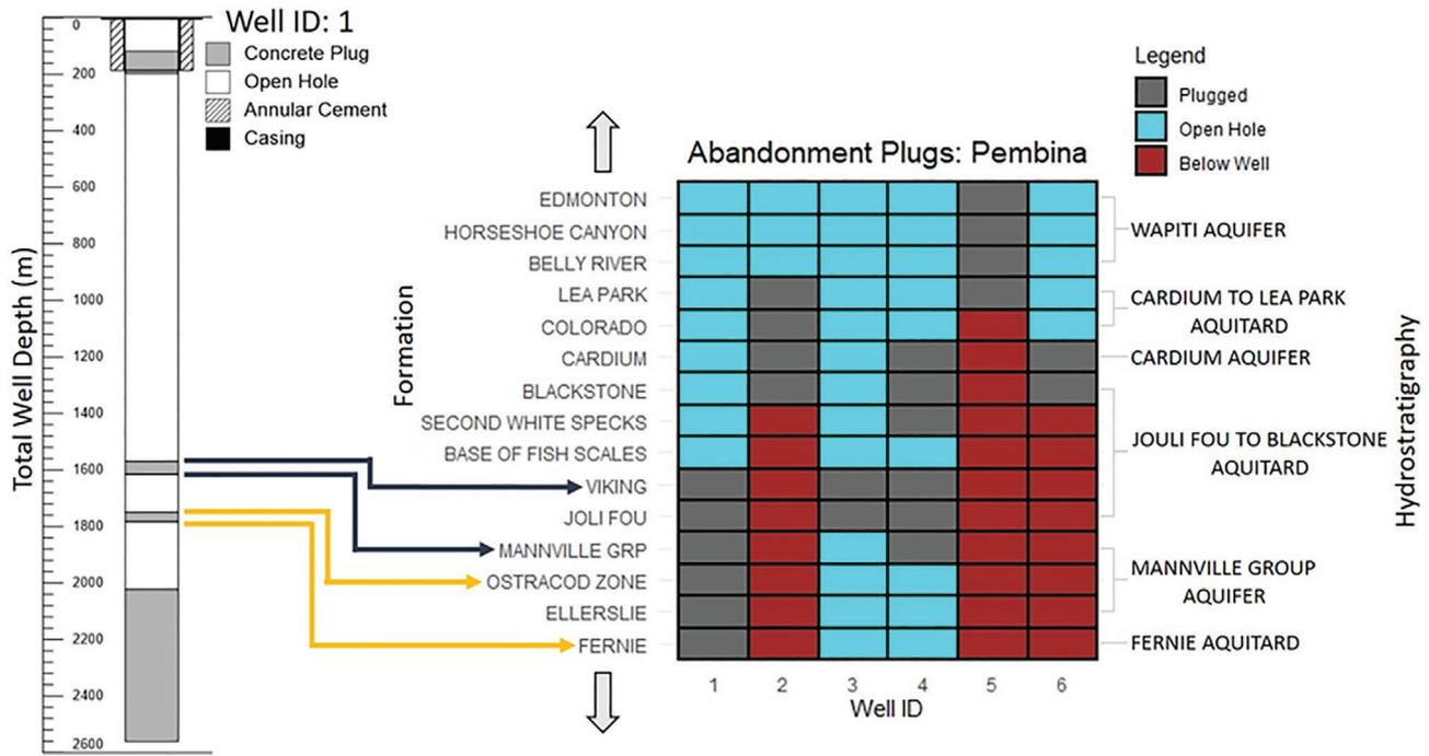
**Figure 7. An example of a typical well abandonment schematic for a drilled and abandoned well on the left with plug placements in old abandoned wells on the right for the Pembina study area.**
