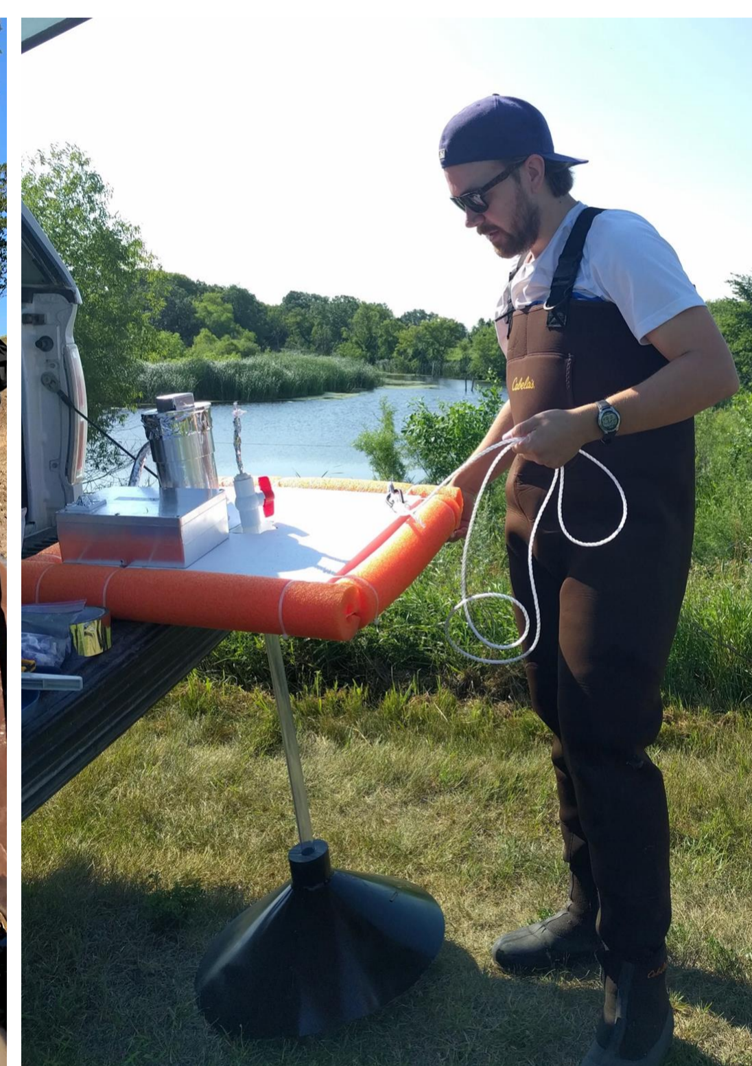
Figure 4: Automated sensor for measuring gas bubbles released from sediments (ebullition) (Photo R.Helmle).
