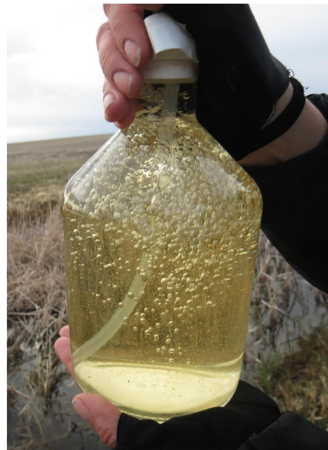
Figure 1: Dissolved gas sampling, headspace equilibrium method.
