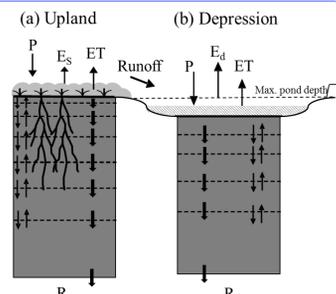
Figure 2 – Conceptual framework of VSMB-DUS model
